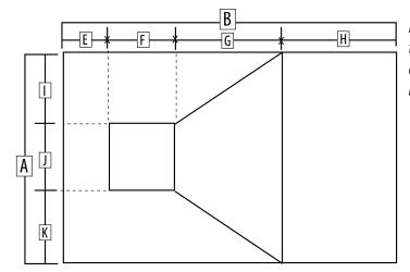
Note: Simply make a chalk mark on the deck at each transition point and measure the distance between each point and record the measurement in STEP 6 on the measuring form.
