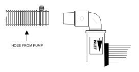
With the clamp in place, push and twist the hose onto the hose barb labeled 'inlet' on your Solar Bear solar heater. Tighten clamp. NOTE: You may need to warm the end of the hose to make it more pliable. This can be accomplished by placing it in hot water for several seconds. 3. Place the loose hose clamp over the new hose. Push and twist the new hose onto the solar heater's 'outlet' hose barb. Secure the clamp firmly, but do not over tighten.
