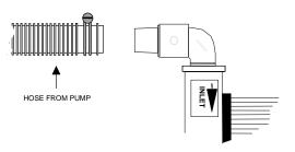
With the clamp in place, push and twist the hose onto the hose barb labeled 'inlet' on your Solar Bear solar heater. Tighten clamp. NOTE: You may need to warm the end of the hose to make it more pliable. This can be accomplished by placing it in hot water for several seconds. 3. Place the loose hose clamp over the new hose (supplied). Push and twist the new hose onto the solar heater's 'outlet' hose barb. Secure the clamp firmly, but do not over tighten.
