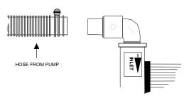
With the clamp in place, push and twist the hose onto the hose barb labeled 'inlet' on your Solar Bear solar heater. Tighten clamp. NOTE: You may need to warm the end of the hose to make it more pliable. This can be accomplished by placing it in hot water for several seconds.
